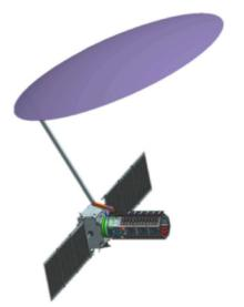
Figure 1. Artist's concept of NISAR spacecraft in flight configuration. Spacecraft velocity vector would be aligned with the long axis of the solar arrays. The L-band and S-band radar electronics are mounted on the octagonal structure pointing to the right.
