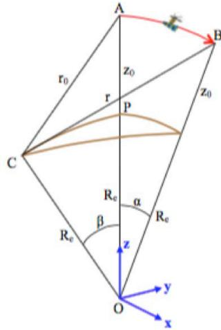
We derived the effective velocity for the point P (directly under the satellite) in Handout 22. The relative height history  $z(t)$  between the point P and the satellite can be written as:
