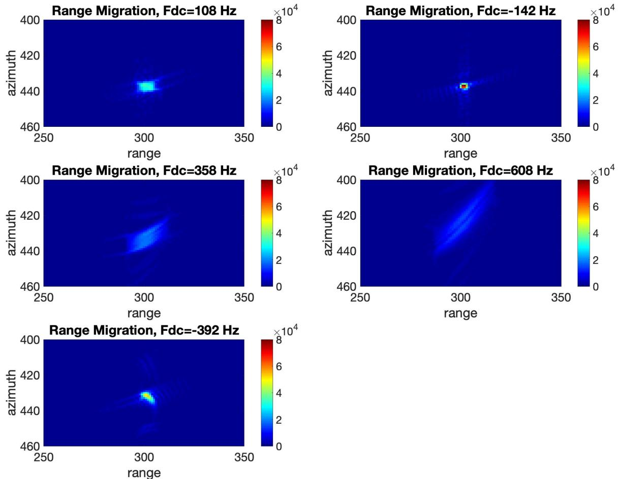
Using the cut and paste algorithm, we get the best concentration of the returned signal with a doppler centroid of -142 Hz. The others have a significant smearing of the returned energy. However, note that our returned signal using the cut-and-paste is still not perfect. We would likely see better results if we also added an interpolation to our cut-and-paste algorithm. Also note that the range migration process increased the sensitivity to the Doppler Centroid ambiguity.
