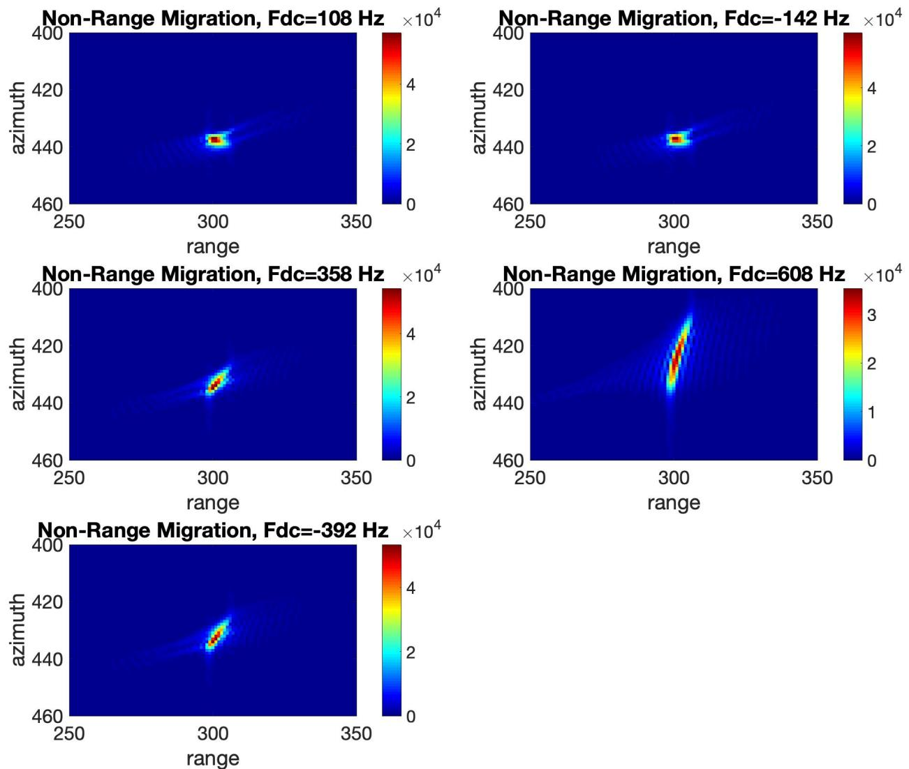
Although the point looks pretty good when zoomed out far, when we zoom in we can see some significant blurring, or spreading out of the signal over range bins. The best response is when we use a doppler centroid of -142 Hz, although our original pick of 108 Hz does almost just as well. 608 Hz does the worst, since it has the most smearing.
