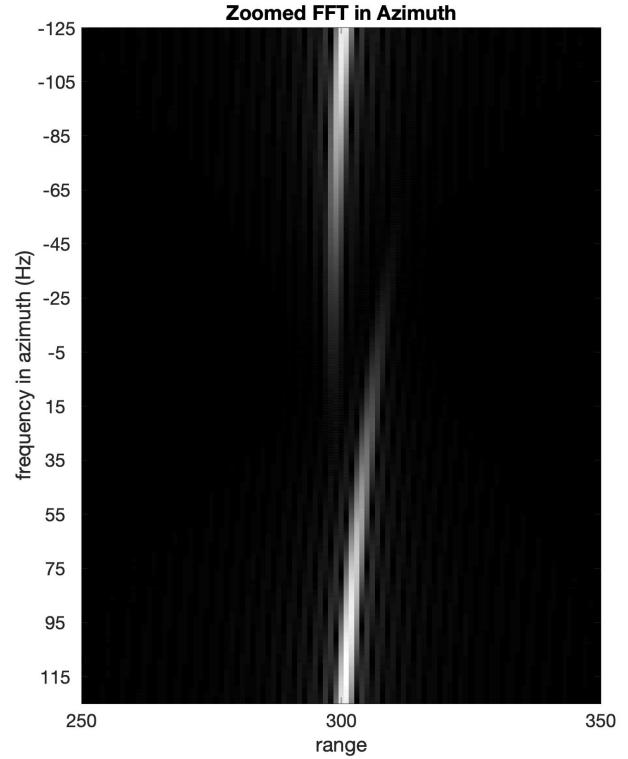
After transforming the range compressed data in the azimuth direction (left), we still see range migration between the two tail ends of the spectra (about 15-20 pixels), especially when we zoom in on range bins 250-350 (right). Notice that fDC is around prf/2 (part c), which explains why the "ends" of the spectra come together around -10 Hz. Also, the azimuth frequency range can have an ambiguity of  $n \cdot prf$ , so we only plot the axis label as [-prf/2 prf/2].
