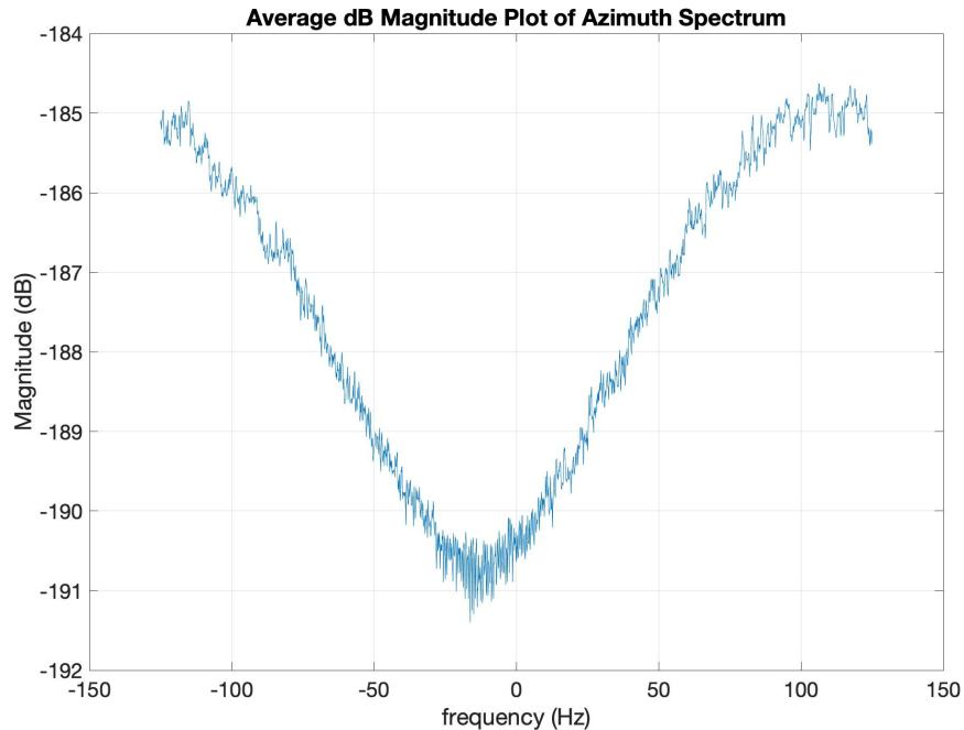
Since we really only have one scatterer, the average phase shift method couldn't be effectively used. Therefore, I estimated the Doppler centroid by finding the peak of the average spectrum and decided on  $F_{DC} = 106$ . To account for the ambiguity, I also added and subtracted multiples of the PRF=250 Hz. Some of the possible  $F_{DC}$  values are:
