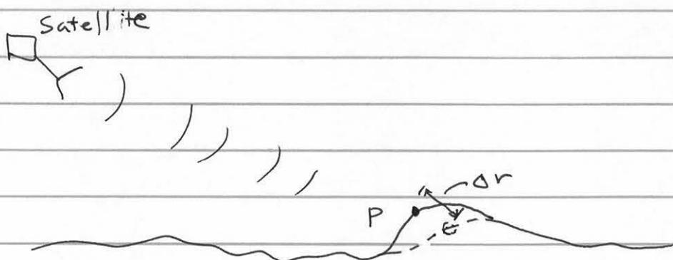
Something has deformed the surface in the vicinity of P and caused it to be closer to the radar at new time  $t_1 = t_0 + \Delta t$ . The phase of the pixel in the two scenes is
