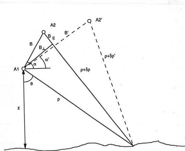
**Figure 1.** Radar imaging geometry. The solid lines show that radar signal paths for the first interferogram pair formed by antennas at A1 and A2. Dashed lines show signal path for second interferogram acquired over the same site but with antennas located at A1 and A2'.
