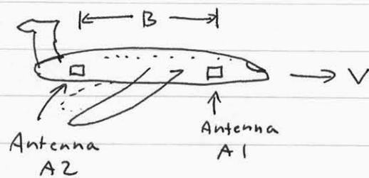
The radar antennas A1 and A2 are mounted on the front and back sections of an aircraft's fuselage, rather than across-track. We will form two radar images again, as we did in the earlier interferometer.
