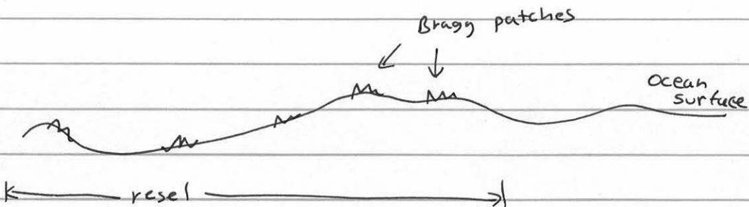
Each patch consists of a few cycles of wavelets with the Bragg condition
