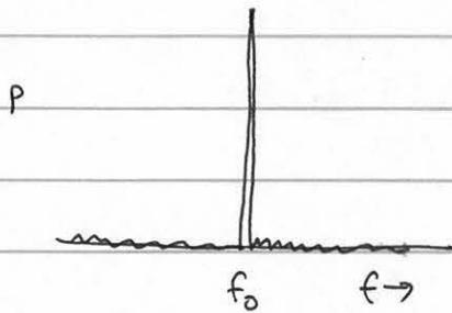
Now suppose we are looking at a series of swell or a fixed current. The entire spectrum will be Doppler shifted to reflect the motion toward the radar.
