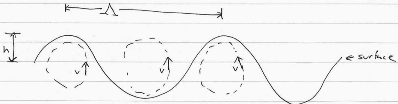
For large-scale ocean waves, called gravity waves because gravity forms the restoring force, we can relate orbital motion to wavelength by considering basic wave equations:
