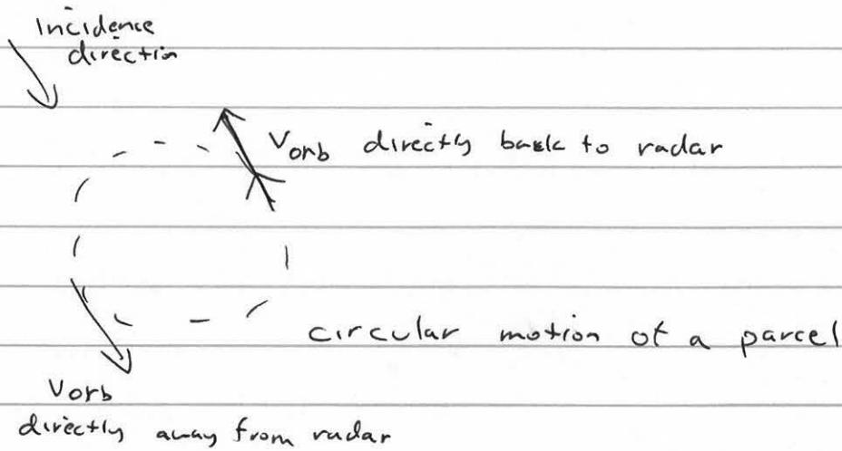
Now, since we can find  $V_{orb}$  directly from the interferogram phase, and  $\Delta$  from the intensity image or phase, we can solve for  $h$ , the height of the swell. Hence using an interferometer for ocean remote sensing characterizes swell nicely.
