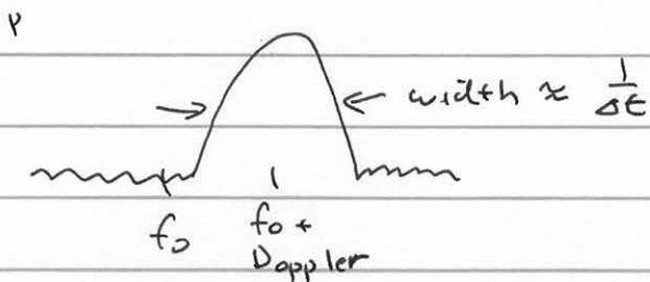
Such measurements seem to indicate lifetimes of  $\sim \frac{1}{2}$  sec for L band,  $\sim 0.1$  sec for C-band for nominally smooth ocean states. It would decrease for rougher seas.
