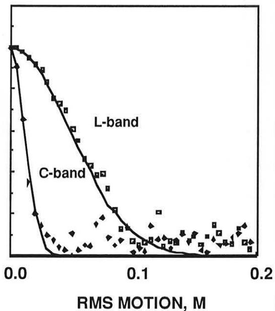
Finally, here is an observed determination of temporal decorrelation at L-band:
