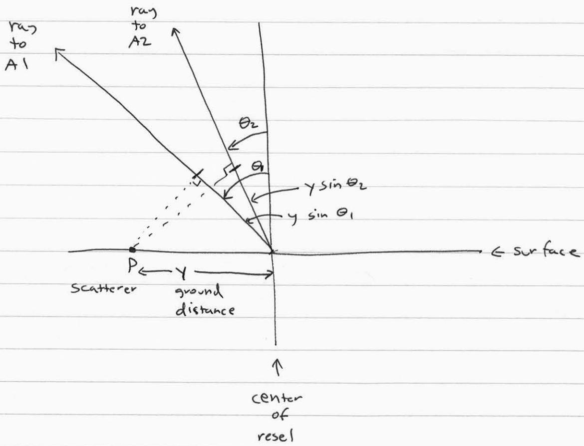
Consider the phase of the reflection from P as compared to the reflection from the center of the resel. The phase from P is advanced by  $y \sin \theta_i$  for the two antennas. If we model the total signal  $s_1$  at antenna 1 as the integral over all of the resolution element, then
