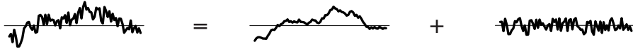
Figure 15.5: Two-scale model with facets. Rough surface is decomposed into two components: (i) a large-scale facet model that describes the overall shape of the surface plus (ii) a small-scale roughness component with low values of residual amplitude.
