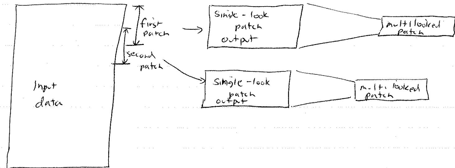
Note the offset from patch to patch in the input data set is less than the patch size. The offset is determined by the number of valid data samples.
