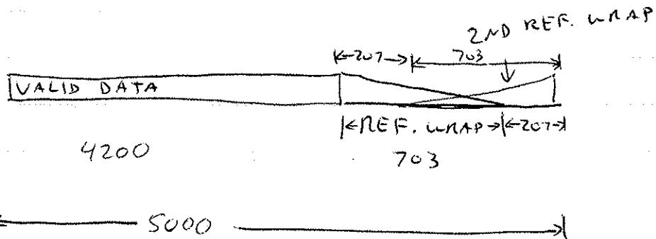
Note that this means we need to transform only the length of the original echo,  $N_{\text{valid}} + N_{\text{ref}}$ , rounded up to  $2^n$  for most ffts, in most cases.
