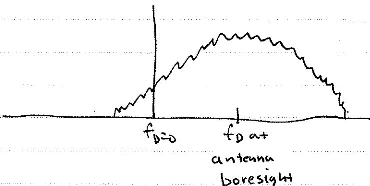
In this case the energy peaks up at a positive value of  $f_D$ . If we measure the centroid of this curve, we can solve
