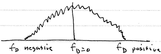
Note the peak at  $f_D=0$  as the antenna boresight is set at 0 radians. As we examine other scatterers the total power falls off as we approach the edges of the antenna beam.
