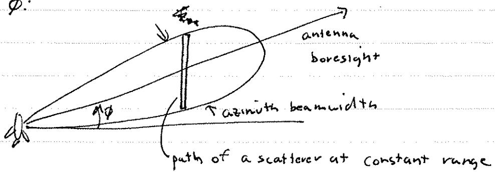
Consider in more detail the path traveled by a scatterer as the plane flies by with this skewed geometry:
