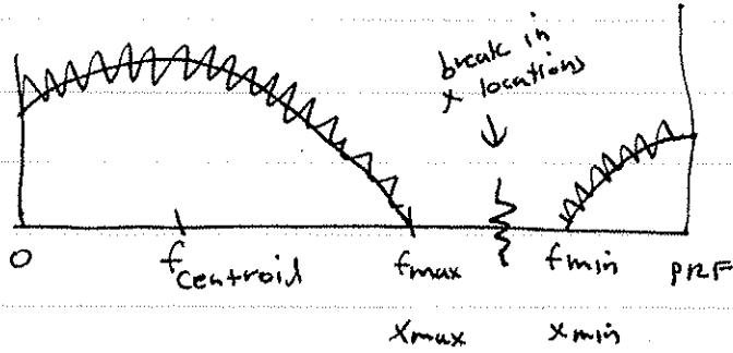
The image here is in two pieces which must be put together to form the full patch without any discontinuities.
