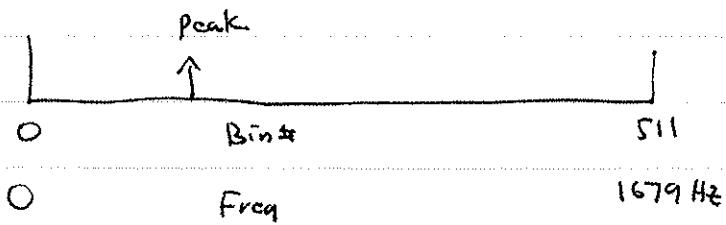
The ~~freq~~ total frequency span is 1679 Hz, so  $\Delta f = 3.28 \text{ Hz/bin}$  and the centroid would be 328 Hz.
