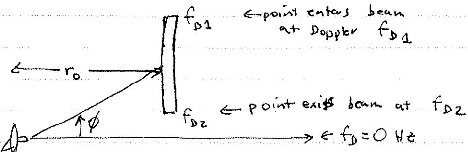
Thus at any instant in time the return in range bin  $r_0$  contains scatterers ranging in Doppler frequency from  $f_{D2}$  to  $f_{D1}$ , which may or may not contain the broadside point at  $f_D = 0$ .
