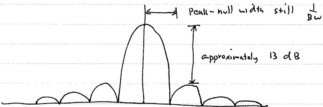
We can calculate the height of the first sidelobe for an ideal sinc function:
