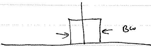
We can describe this function as  $\text{rect}\left(\frac{f}{BW}\right)$ , a rectangle function, centred at 0, of width BW. Remember that it transforms into a sinc function:
