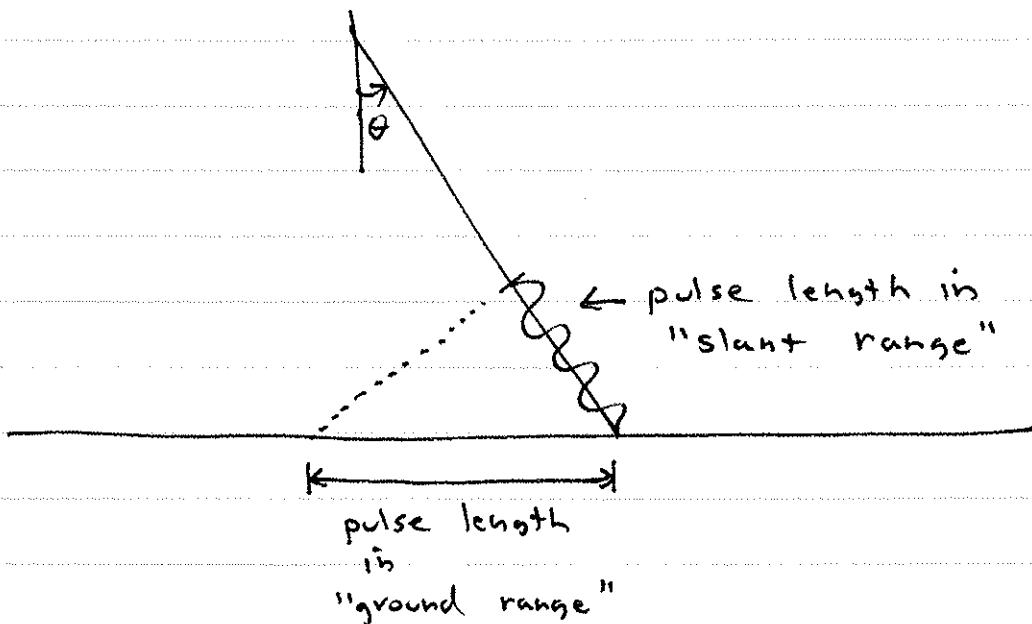
For a pulse length  $\tau$  in time the "length" in meters is
