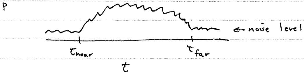
So the impulse transmit pulse is spread out over a range of times. If instead we were to transmit a pulse of finite duration, each point on the ground would return a duplicate of the transmit pulse, properly scaled in amplitude according to its reflectivity, propagation losses, and antenna weighting.
