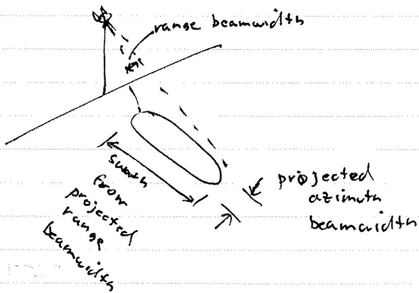
If the antenna size is  $l \times w$  meters, the distance to the center of the swath  $r$ , and the look angle  $\Theta$ , we had
