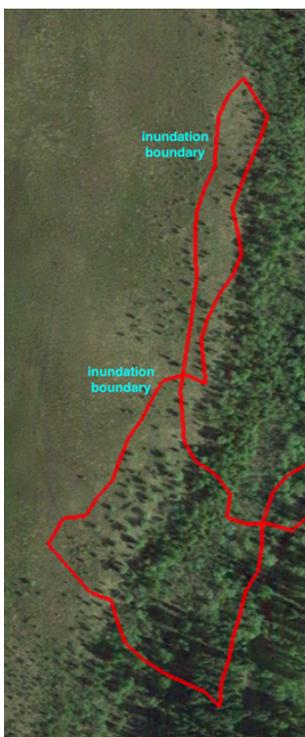
Figure 8-16. Using GPS tracking (red line) to delineate inundation extent. Bonanza Creek wetland area, Alaska, June 2017, visualized in google earth image obtained when the area was not flooded.
