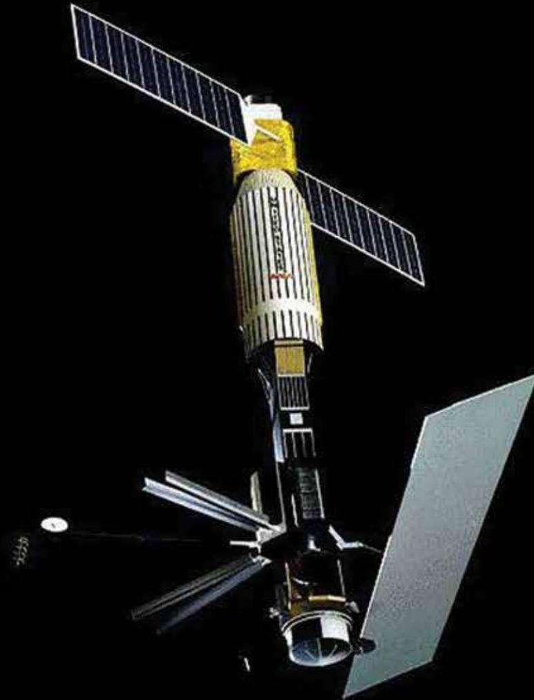
The first civilian SAR satellite in history, called SEASAT, was launched by NASA in 1978. SEASAT's L-band (24 cm wavelength) SAR operated for three months before the failure of the spacecraft's power system. SEASAT led to a series of NASA space shuttle-based radar missions and inspired the development of spaceborne SAR systems worldwide. Launching another free-flying scientific SAR in the U.S. has proven elusive, despite strong demand from the science and applications community.
